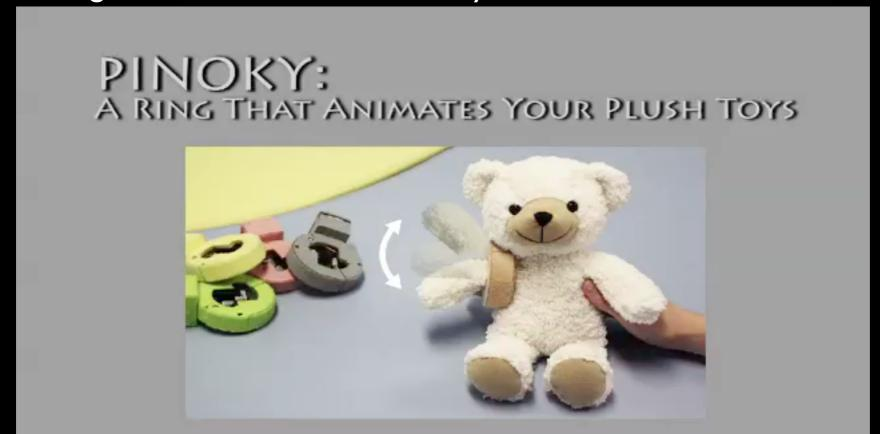
PINOKY is a wireless ring-like device that can be externally attached to any plush toy as an accessory that animates the toy by moving its limbs.
